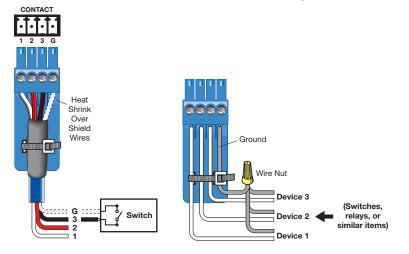
Figure 6. Wiring the Contact Closure Connector
